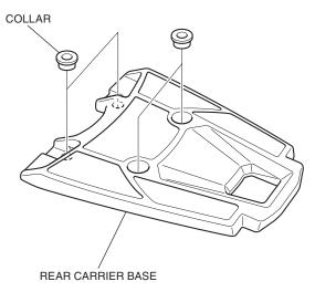
3. Install the rear carrier base as shown.
